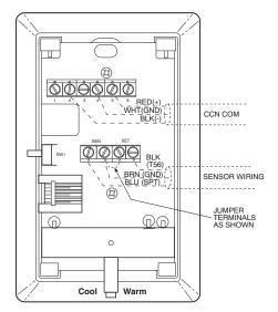
Fig. 45 - T-56 Internal Connections
